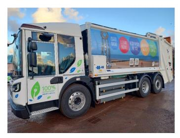
We added two Dennis Eagle e-Collect lorries to the waste collection fleet. Both lorries are used on the county's northern rounds which will include Rhyl, Prestatyn and down to the Trefnant area. They are able to put in up to 100 miles and 1000 bin lifts per single charge.
